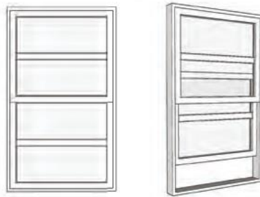
Single Hung Window with Four Horizontal Lights
